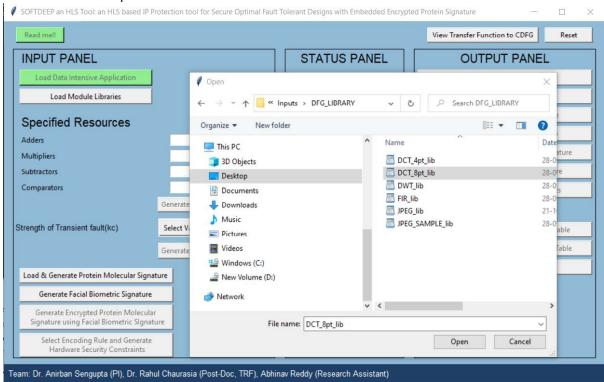
**STEP-4:** Post loading module library (15 nm open cell library) its Tab turns GREEN as shown below. Next, the user is asked to enter/specify the resources based on which design is to be scheduled/generated. *Note:* if user enters the resource configuration exceeding the limits of Min/Max available resources in the module library, then the tool throws an error saying 'Invalid Resource Constraints'. The output screen is shown below:
