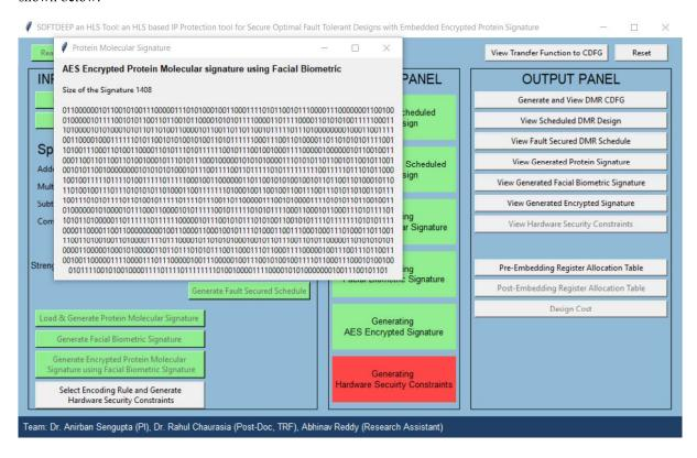
**STEP-9:** Next, user can generate hardware security constraints corresponding to encrypted signature using encoding rule by clicking on Tab' Select Encoding Rule and Generate Hardware Security Constraints'. Post clicking on Tab a pop-up window appears for user to select encoding rules. User can select any of the available encoding rules from the dictionary (for generating covert hardware security constraints) as shown below:
