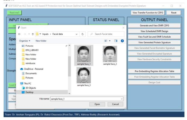
→Post loading the facial image, Tab 'Load Facial Image' turns GREEN as shown below. Next the user enters grid size (e.g., 500X500). Next by clicking Tab 'Generate Facial Features' facial features, features dimensions and their corresponding binarized signature is generated and it turns GREEN and as shown below:
