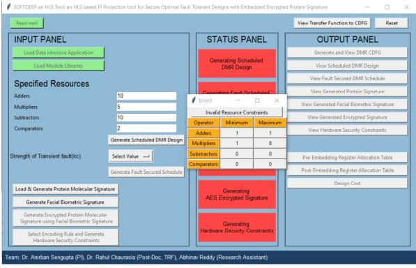
→Now, by entering the resources within the range, user can generate scheduled DMR design. **Post clicking on Tab** 'Generate scheduled DMR Design', the Tabs 'Generate and View DMR CDFG' and 'View Scheduled DMR Design' in the OUTPUT PANEL gets enabled and the status bar 'Generating Scheduled DMR Design' turns GREEN.
