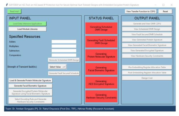
→Next, the user is asked to load module libraries. By clicking the Tab 'Load Module Libraries' a pop-up window appears for user to select corresponding module library which comprises the details of hardware functional unit (FU) resources such as multipliers and adders/subtractors (in terms of area and latency of resources) and available hardware resources for allocation. *Note: For example, library corresponding to DCT\_8pt\_benchmak has been selected here.* The output screen is shown below:
