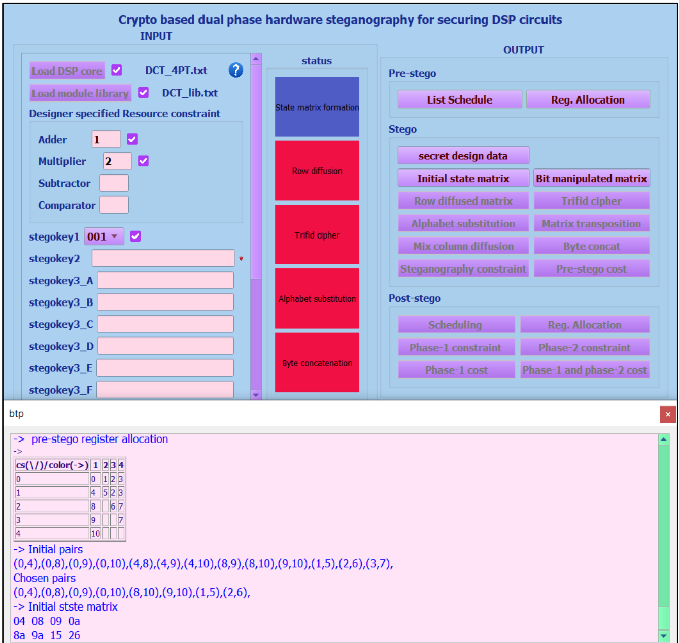
Fig. 13. Snapshot of the tool after feeding DFG of 4-point DCT, resource constraints and stego-key1; the output window is shown in the lower portion
