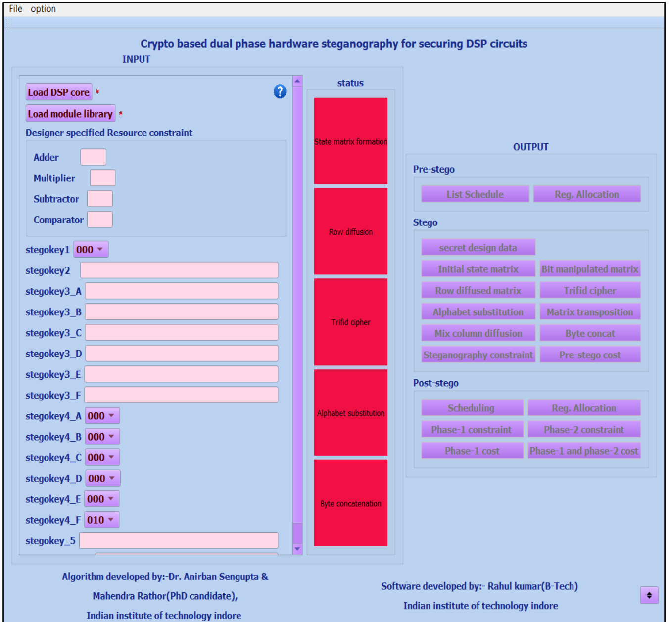
Fig. 12. A snapshot of the GUI of crypto-stego tool for DSP hardware accelerators
